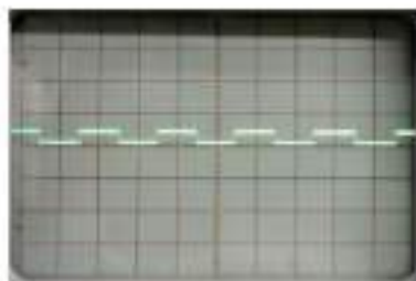
Output of Detector circuit (CH1-2V/div; TB- 0.5mS)
