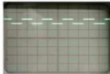
Input to Emitter LED (CH1-5V/div; TB- 0.5mS)
