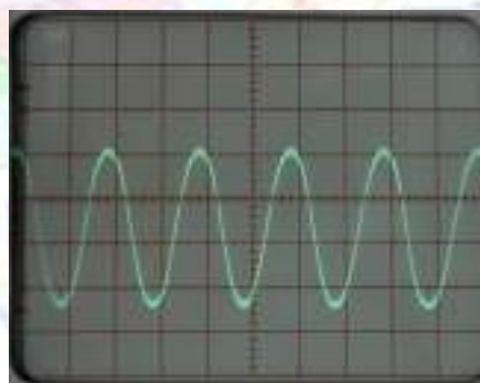
Detector output (after bending)(CH1-0.1V/div; TB- 0.5mS)
