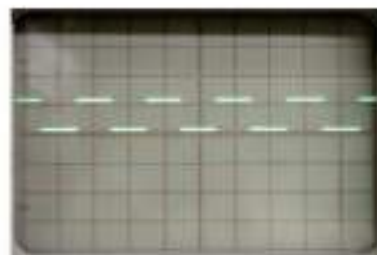
Output of Comparator circuit (CH1-5V/div; TB- 0.5mS)
