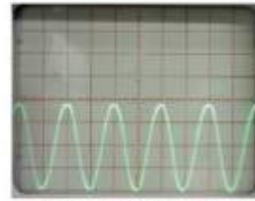
Output of AC Amplifier circuit (CH1-2V/div; TB- 0.5mS)
