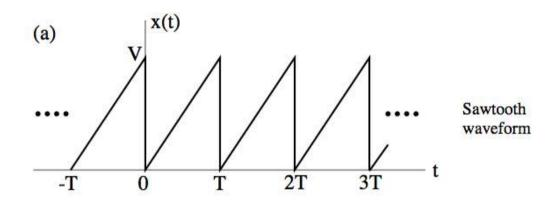
**Result:-** Generating the sawtooth wave with different amplitudes and frequencies.
