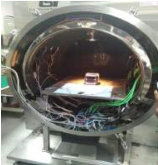
Satellite Chief Ashhar Farhan is Testing the CUBESAT in a chamber
