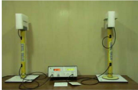
Overall setup, with receiving antenna mounted for making E-Plane measurements.
