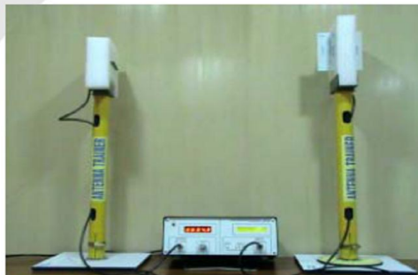
Overall setup, with receiving antenna mounted for making H-Plane measurements.
